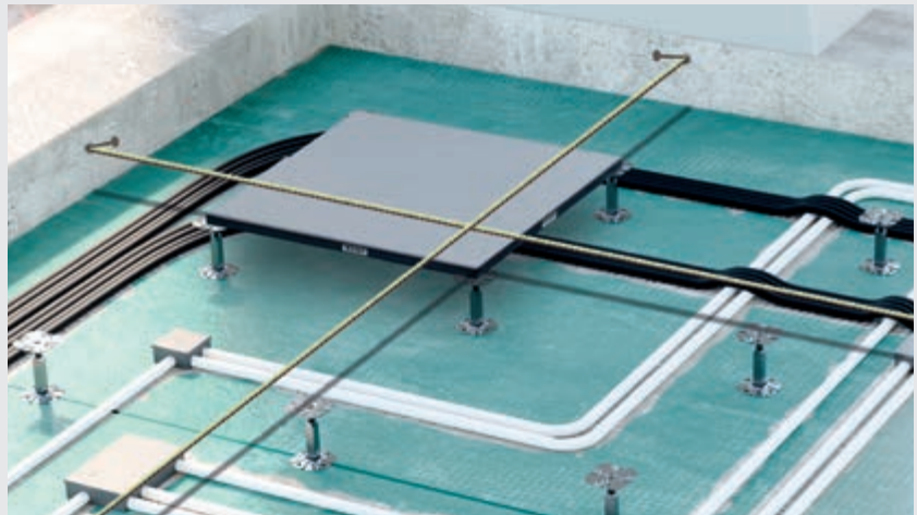
Positioning the first panel using the two orthogonal wires
