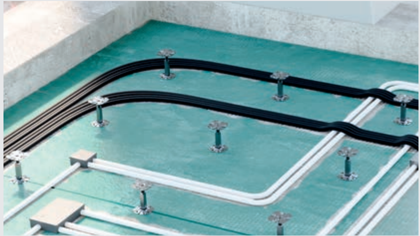
Positioning of columns
