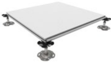
TETRIS FLOOR partially accessible floor with tongue and groove interlocking system
